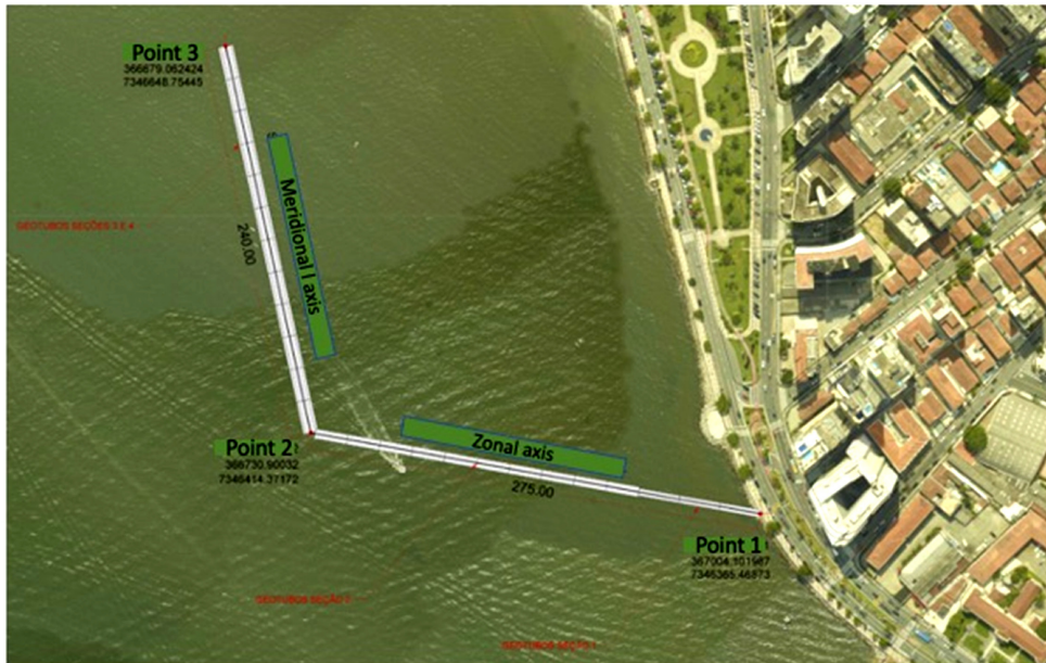
Figure 5. Detail of the Pilot Project for mitigation and monitoring Ponta da Praia erosion processes showing the main zonal and meridional axis with the submerged breakwaters (Source: GARCIA & GIRELI 2019).
